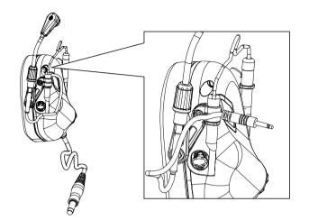
Step 2: Rotate the slider perpendicular to the earcups as illustrated. Press thumb against the junction of slider and earcups, and pull outwards with force to seperate.
