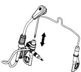
Step 5: Pinch the rubber end and pull it outwards, and then detach the microphone arm from slider.
