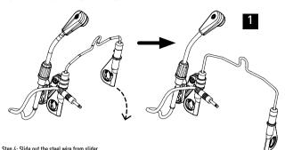
Step 4: Slide out the steel wire from slider
